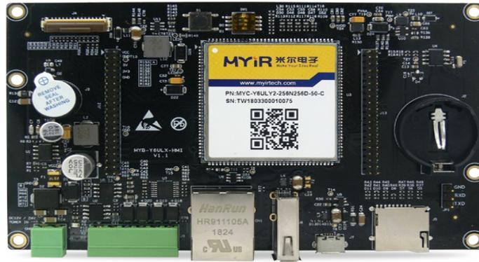
Figure2-2 MYD-Y6ULX-HMI top view
